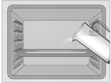
3. Set the oven to easy steam cleaning mode and run at 100°C for 15 minutes.
