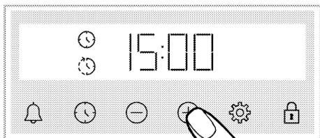
» After the cooking end time is set, the symbol and the symbol will appear constantly on the display. As soon as cooking starts, the symbol disappears.
