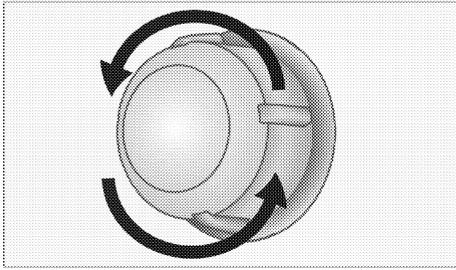
3. If your oven lamp is type (A) shown in the figure below, rotate the oven lamp as shown in the figure and replace it with a new one. If type (B) is a model, pull it out as shown in the figure and replace it with a new one.
