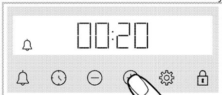
» After setting the alarm time, the
