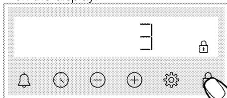
» The symbol appears and the 3-2-1 countdown begins on the display. When the countdown is over, the key lock is activated. When any key is touched when the key lock is set, the timer sounds an audible signal and the symbol flashes.
